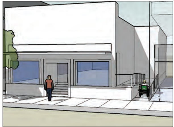
Figures 7.2 and 7.3: External wheelchair ramps accessed directly from sidewalk to ensure easy access. Ramps are located on the side of building (illustrative images).
